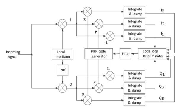
Figure 2 Delay Lock Loop (DLL) block diagram with six correlators
