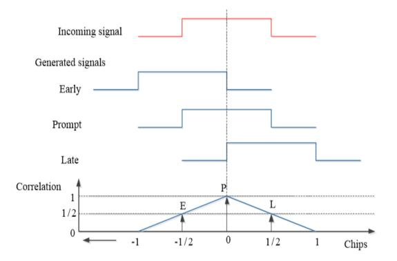
Figure 1 A perfectly tuned code loop with highest correlation at prompt output
